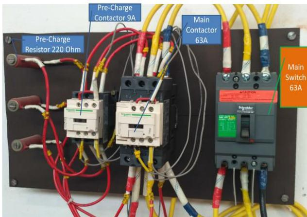
Figure-6. Hardware model of pre-charge circuit.
