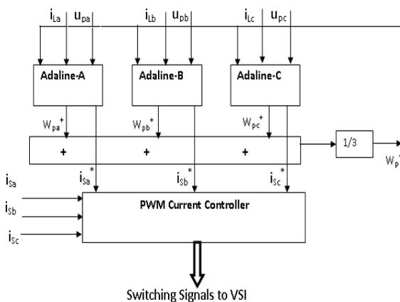
Figure-8. ADALINE control block diagram.
