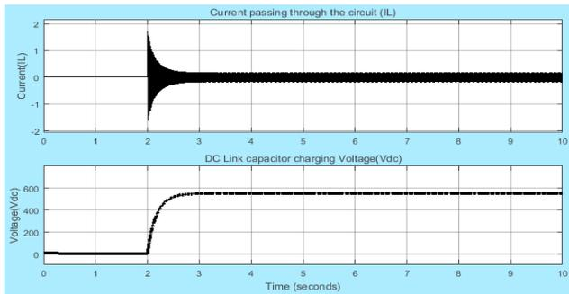
Figure-5. Charging of capacitor with a delay of 2 Sec.
