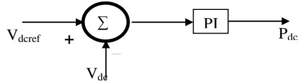
Figure-9. Conventional DC link voltage controller.
