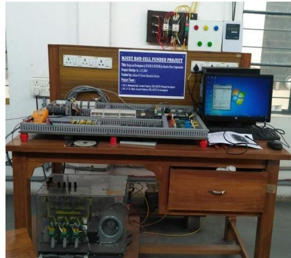
Figure-11. Complete test setup model of DSTATCOM.
