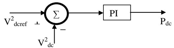
Figure-10. Fast acting DC link voltage controller.
