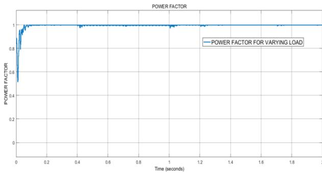
**Figure-19.** Power factor of varying load with controller showing UPF.
