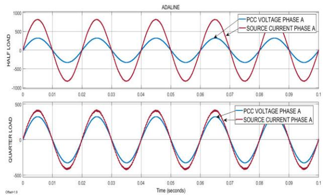
**Figure-21.** Wave form of the voltage and current of phase a with ADALINE controller.
