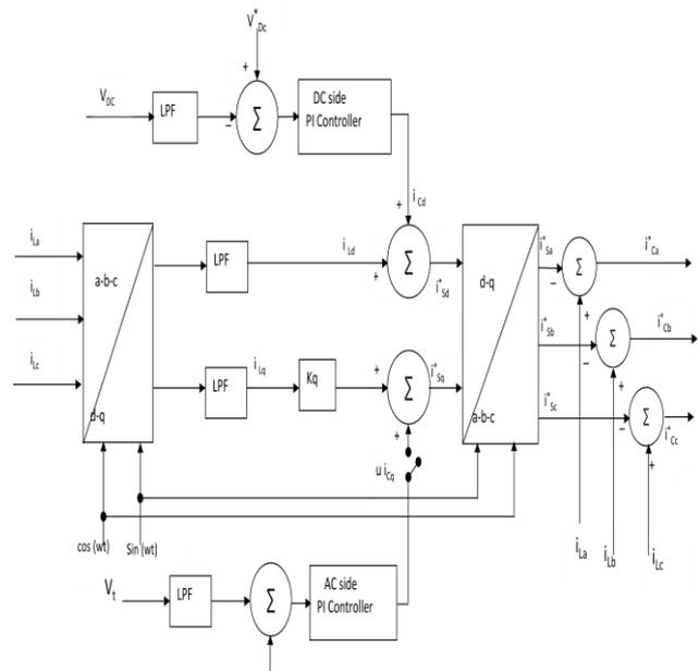
Figure-7. SRF control block diagram.
