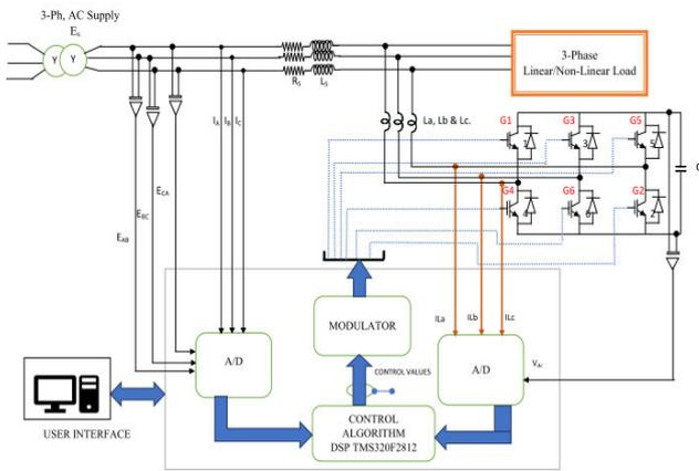
Figure-13. Complete hardware diagram of DSTATCOM.
