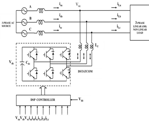
Figure-1. Basic building control block diagram of D-STATCOM.
