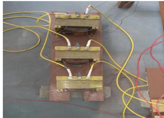
Figure-3. Inter phasing inductor.
