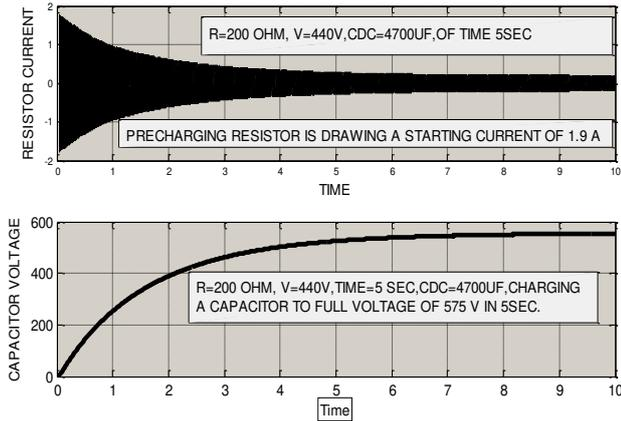
Figure-4. Charging of capacitor with out delay.
