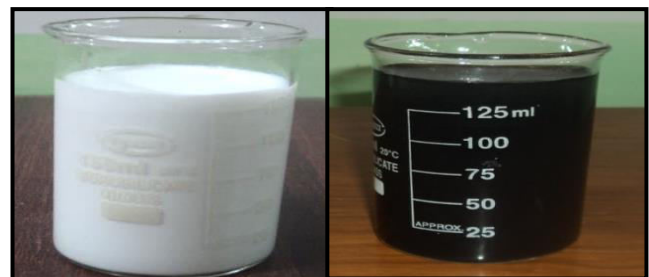
Figure-1. Hybrid Nano fluid copper Cu (25nm) + Aluminum Al (25nm) and Aluminum oxide Al 2 O 3 (50nm) + titanium oxide TiO 2 (50nm).
