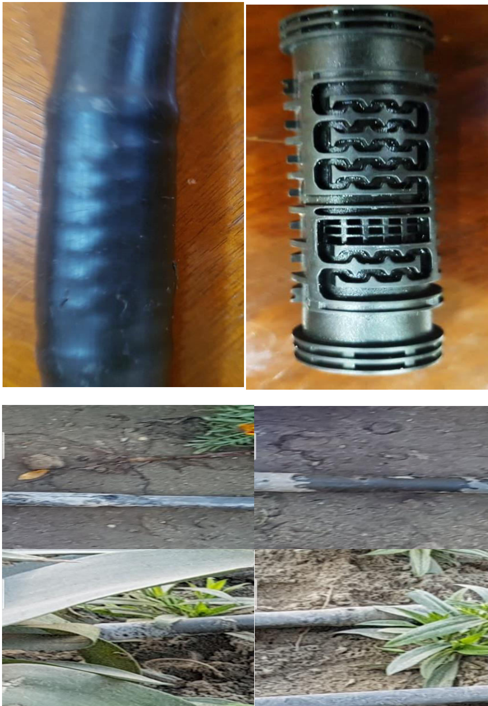
Figure-7. A. The produced pipe according to the control system during and after the perforation used in the experimental Study, B. The produced pipes and used in the irrigation systems.
