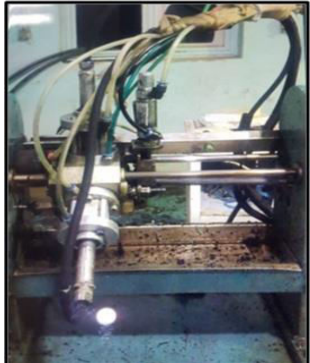
Figure-4. The perforation unit used to production the drippers.
