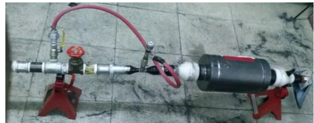
Figure-6. Portion of real diesel particulate arrestor test apparatus.
