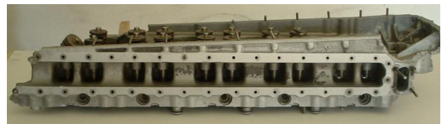
Figure-2. The head "A" after disassembly and cleaning (air intake side).
