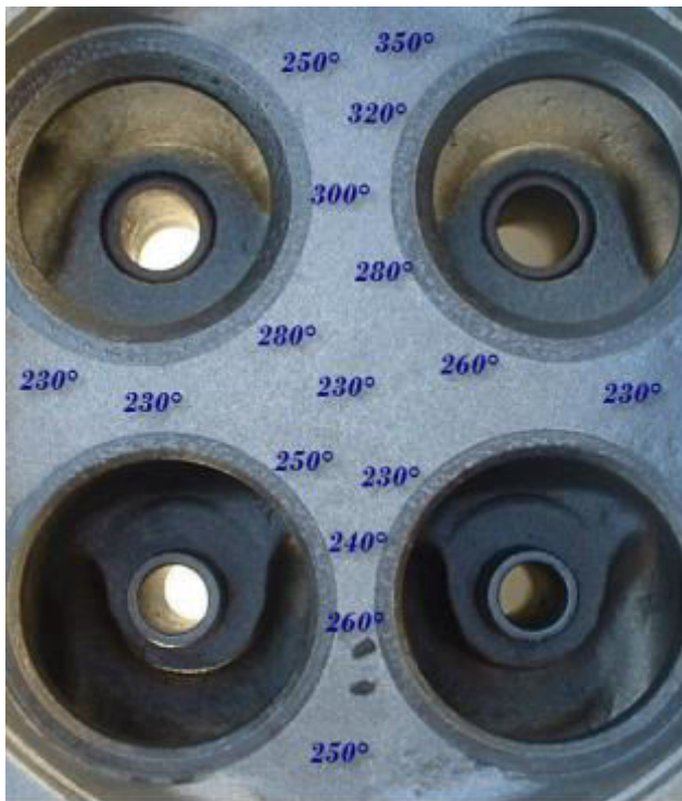
Figure-7. Temperatures (Degree C). Intake valves below (smaller valve guides).
