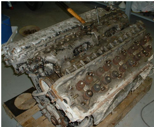
Figure-1. The Mosquito port RR Merlin XX engine at the beginning of the disassembly in Forli Laboratory of the Università degli Studi di Bologna - Italy.
