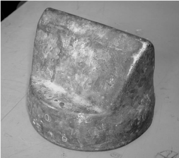
Figure-2. Casting of H11 steel splitter obtained by electric slag chill casting ( \times 0,25 ).
