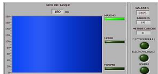
Figure-5. Real-time tank level indicator block
