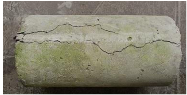
Figure-9. Split tensile testing.
