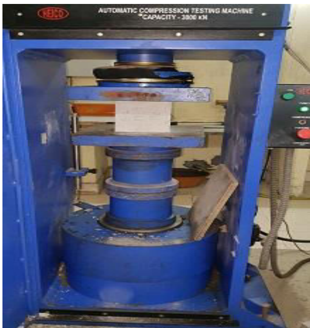
Figure-5. Compressive testing machine.
