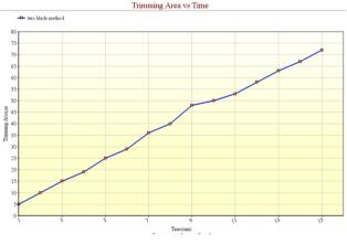
Figure-12. Result of trimming area vs time for two blade method.
