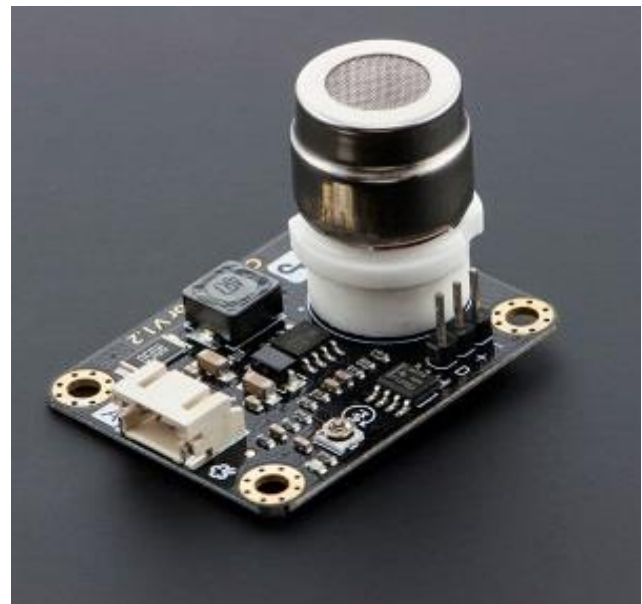
Figure-1. MG811 sensor with sen0159 module (Didacticas electronicas, 2019).
