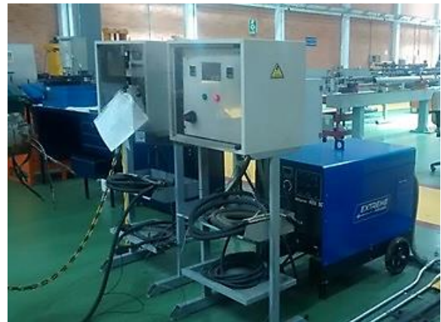
Figure-6. Stator drying machine-implemented.
