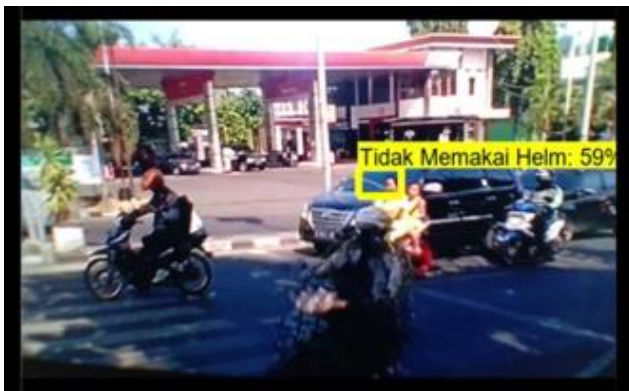
Figure-13. Example of violation detection of not wearing a helmet.
