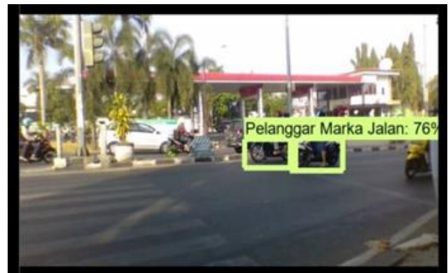
Figure-14. Example of road marking violation detection.
