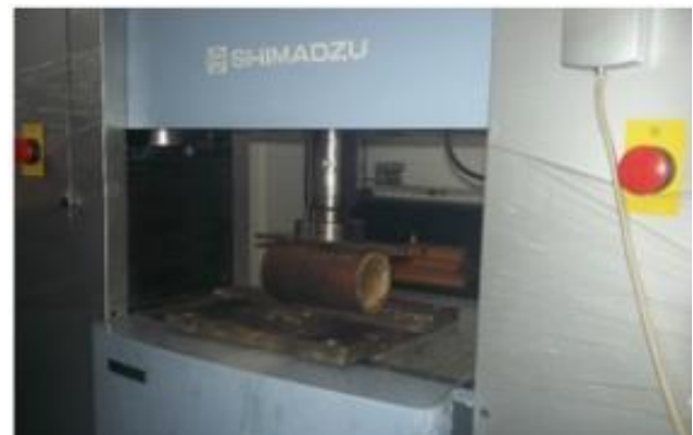
Figure-2. Perpendicular-to-the-fiber compression resistance test.
