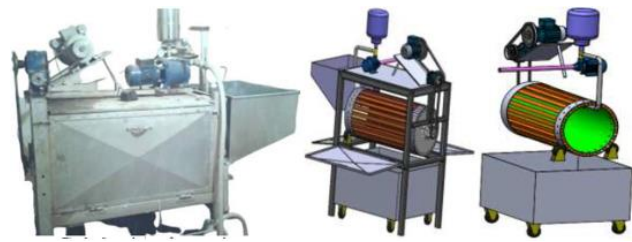
Figure-9. Washing machine for root crops [40].
