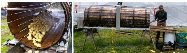
Figure-6. Barrel washer for cleaning root crops [32].
