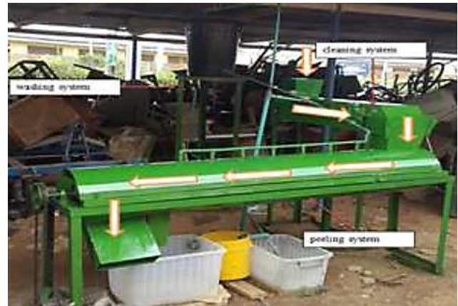
Figure-8. Cassava cleaning, peeling and washing machine [15].
