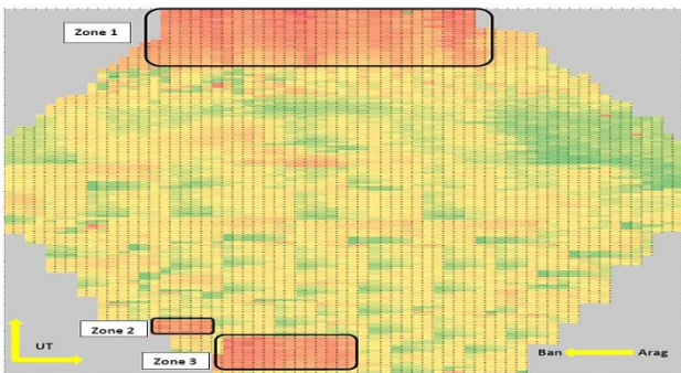
Figure-3. Ultrasonic thickness measurement results.
