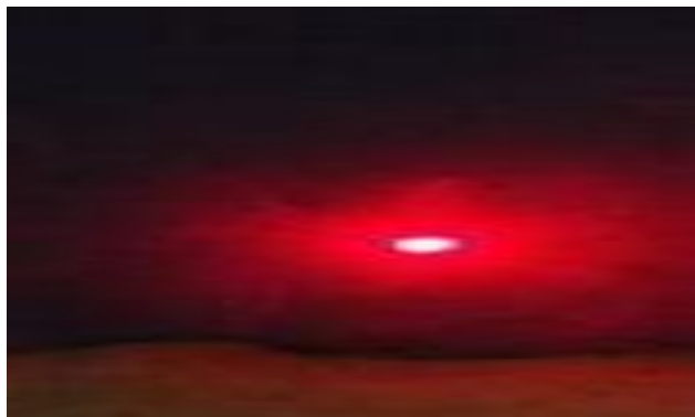
Figure-8. Applying red filter for finding the brightest spot in captured image.
