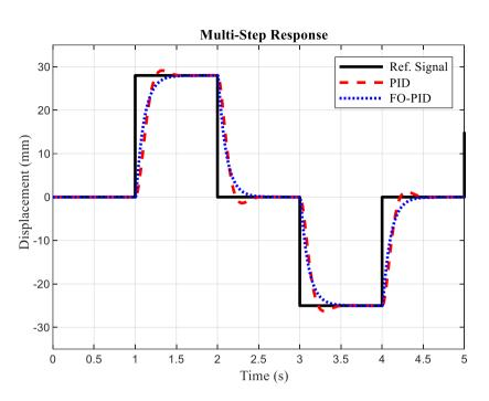
Figure-4. Multiple-step reference response.
