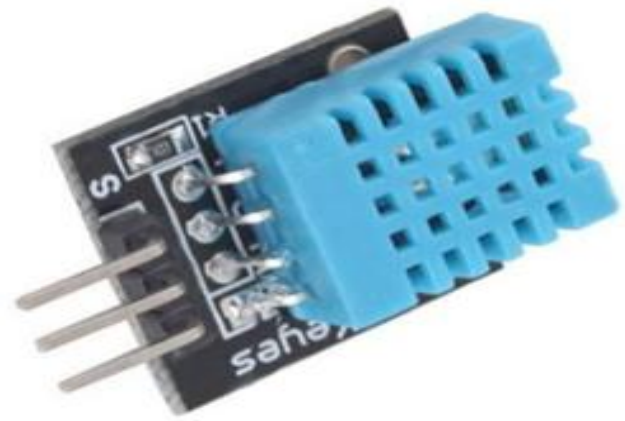
Figure-5. The DHT11 temperature and humidity sensor.
