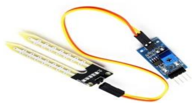
Figure-4. Soil moisture sensor.
