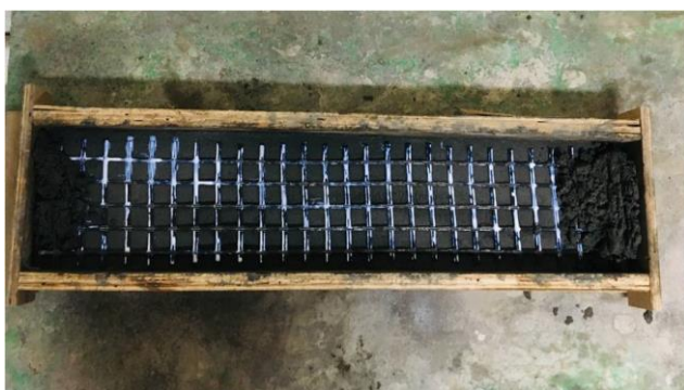
Figure-5. Placing of textile mesh while casting the specimen.
