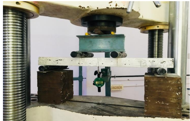
Figure-6. Flexural test setup.
