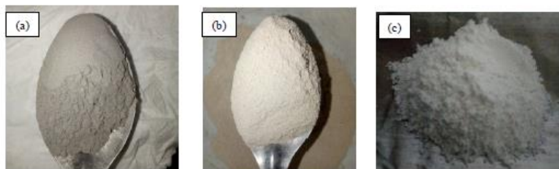
Figure 1. a. Fly ash before calcination, (b) fly ash after calcination and (c) silica precipitation
