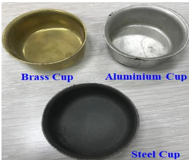
Figure-16. The produced cups (brass, aluminum, and steel).
