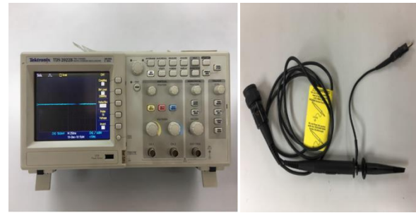
Figure-11. Tektronix TDS 2022B Oscilloscope and its probe
