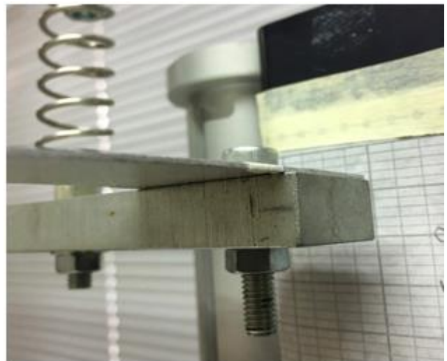
Figure-8. Close-up view on the dynamic absorber-main system mounting
