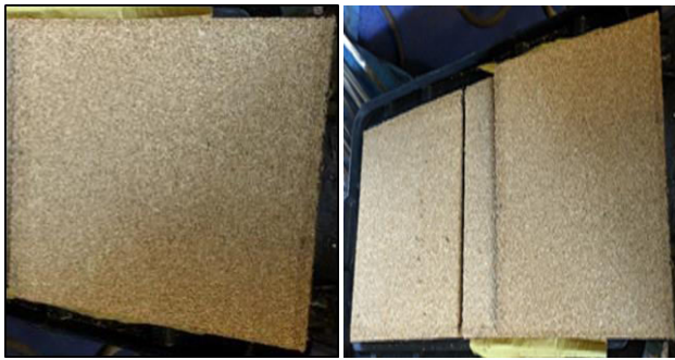
Figure-4. Sample particle board (sawdust: rice husk: starch - 30:55:15).
