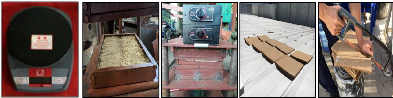
Figure-1. Manufacturing of the particle board.
