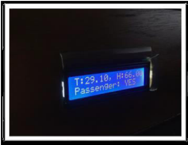
Figure-11. Liquid display crystal show the temperature and presence of the baby.
