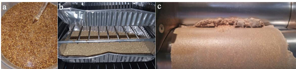
Figure-1. a) PSH, mercerization; b) PHS, drying; c) Compounding of NBR/silica/PSH composites.
