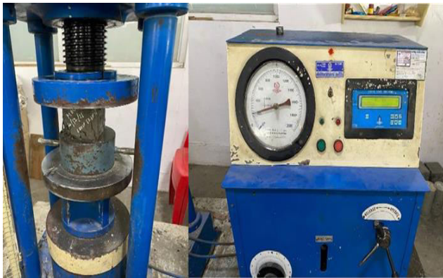
Figure-3. Compression strength test.
