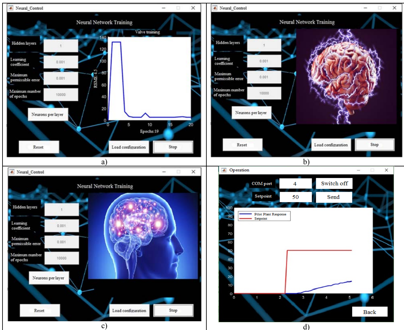
Figure-4. Main screen, a) Training view, b) Main program view loading the selected configuration, c) initial screen view saving the configuration, and d) Operation screen in communication with the module.
