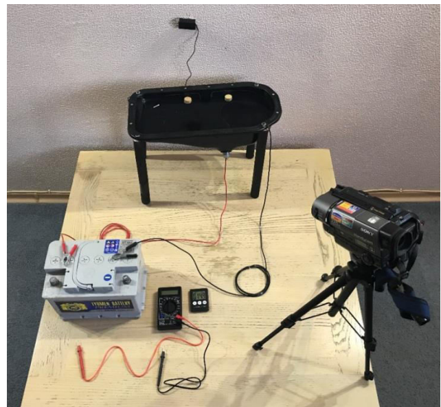
Figure-7. Test bench for electric engine pre-start heaters.
