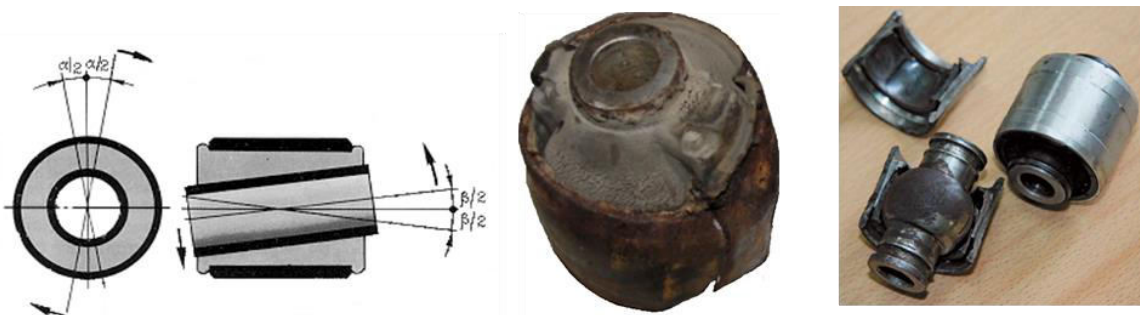
Figure-2. Possible deformation of the rubber bush of the silent block and its destruction.
