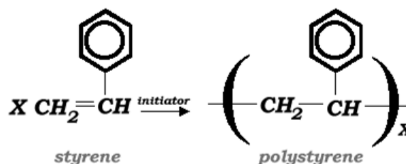
Figure-1. Chemical reaction of polymerization of styrene.
