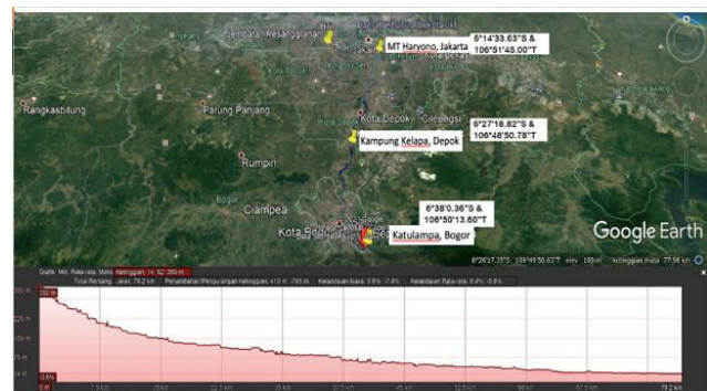
Figure-2. The stretch of the Ciliwung River from Katulampa, Depok to MT Haryono, East Jakarta, with a river length of 79.2 km, with a maximum slope of 3.8%.
