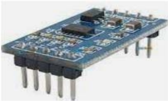
Figure-3. Accelerometer sensor.
