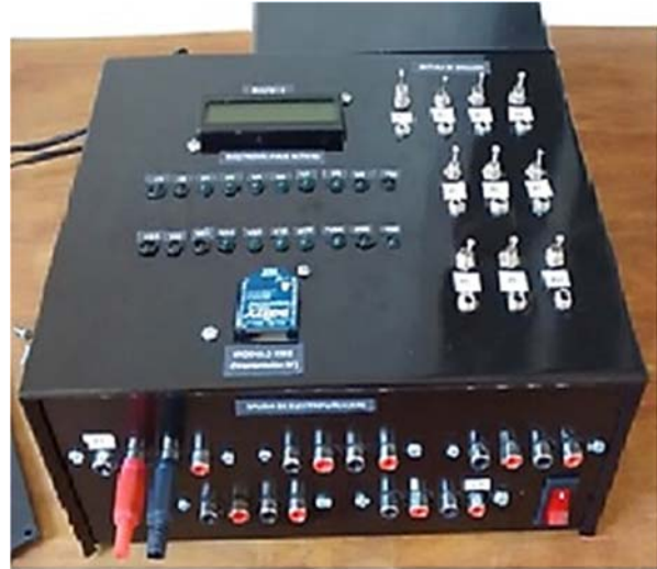
Figure-2. Implemented controller device.
