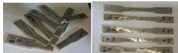
Figure-5. Fracture of the specimen after the tensile test.
