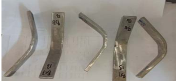
Figure-7. Surface bending test results.
