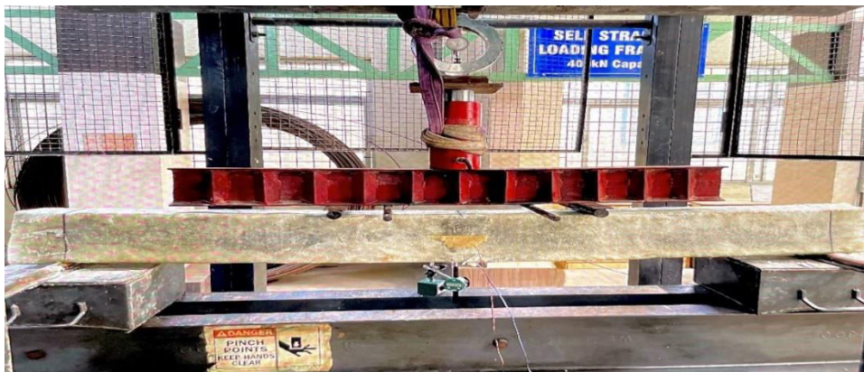
Figure-4. Experimental setup for GFRP wrapped beam.
