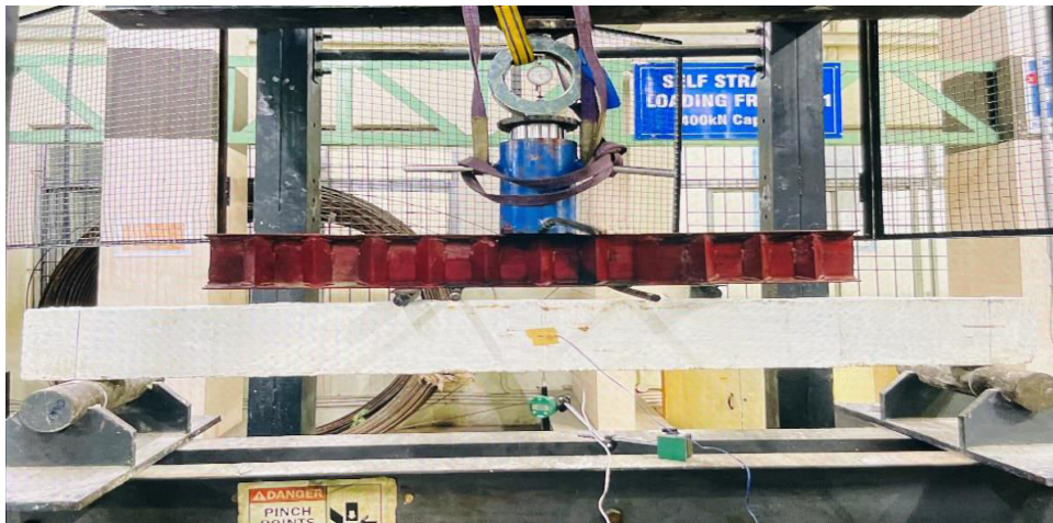
Figure-2. Experimental setup for flexural strength of conventional beam.
