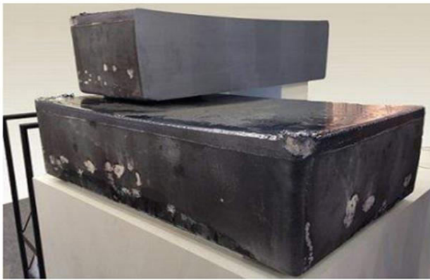
Figure-4. Monolike G6 (600 kg) ingot cut into 2 pieces to show the structure.
