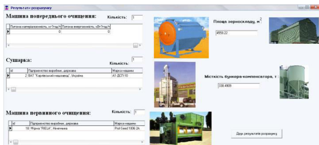
Figure-7. General view of the output interface of a computer program for calculating the composition of the system of post-harvest grain processing machines.
