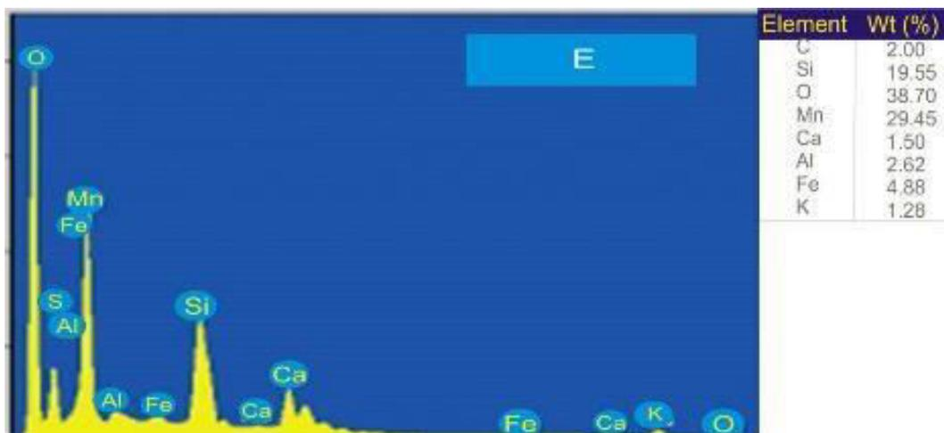
**Figure-3.** EDX micrograph of developed manganese oxide nanoparticles.
