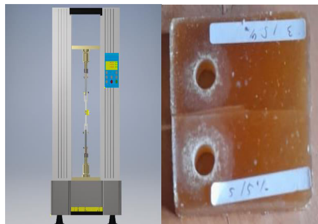
(a) Crack Testing machine (CNT). (b) Molded specimen
