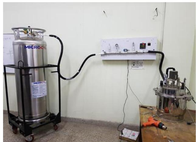
Figure-1. Cryogenic treatment setup.
