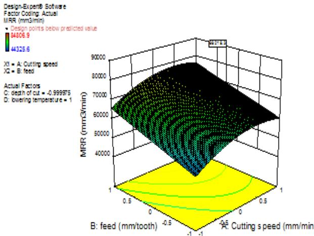
**Figure-3.** Surface plot for variation MRR with CS vs FR.
