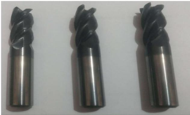
**Figure-2.** Different cryo-treated tools.
