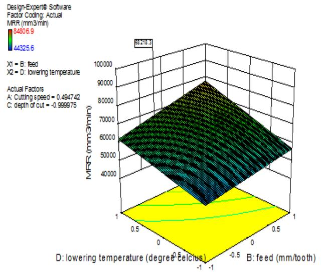
**Figure-4.** Surface plot for variation MRR with lowering temperature vs. feed.
