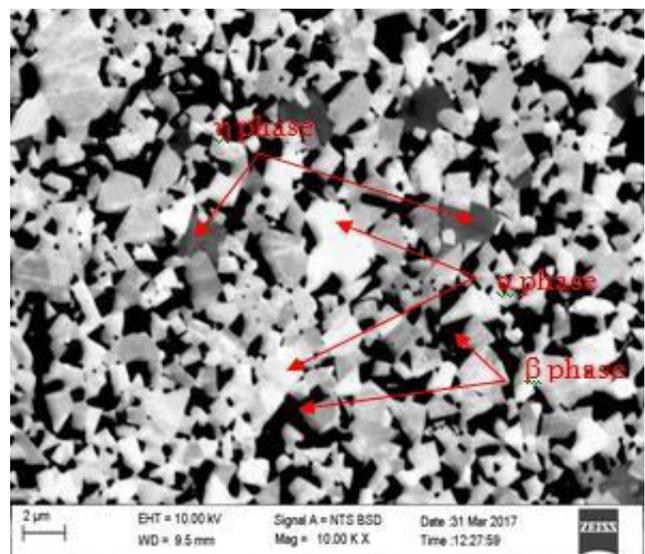
Figure-8. Microstructure of tungsten carbide tools.
