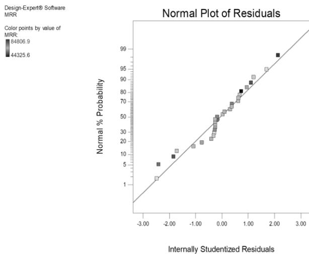
Figure-6. Normal plot of residual for MRR.
