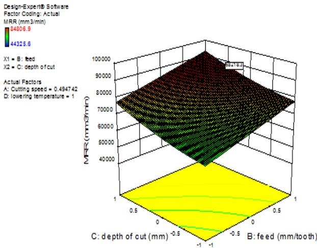
Figure-5. Surface plot for variation MRR with depth of cut and feed.
