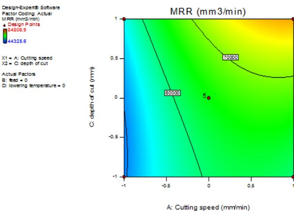
Figure-7. Contour plot for MRR.
