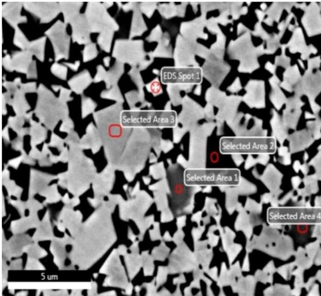
Figure-9. Microstructure of DCT tungsten carbide tools.
