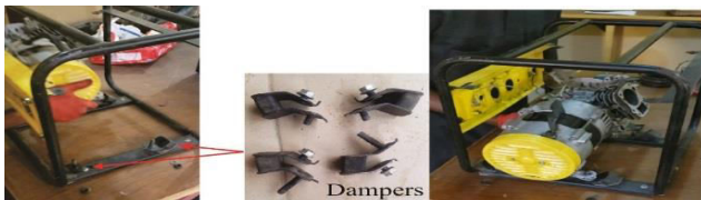
Figure-3.32. Positioning the alternator and crankshaft housing onto the FLG chassis.
