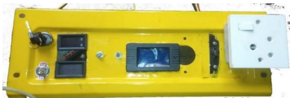
Figure-3.26. Completed FLG control panel.
