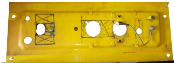
Figure-3.25. FLG control panel showing mark outs and cut-outs.
