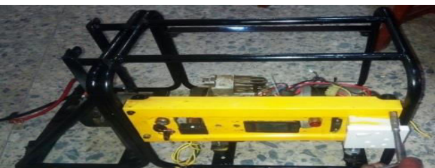
Figure-3.34. Control panel mounted on the FLG chassis.
