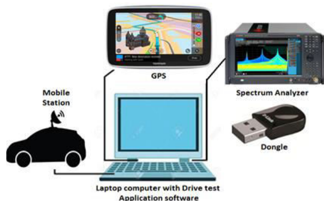
Figure-3. Block diagram of drive test measurement.
