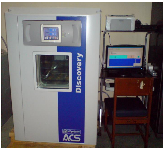
Figure-1. Test chamber with constant temperature and humidity (Model DY110, Angelantoni Asean Pte Ltd., Singapore).
