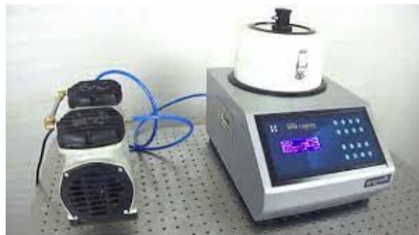
Figure-2. Spin coater device [12].
