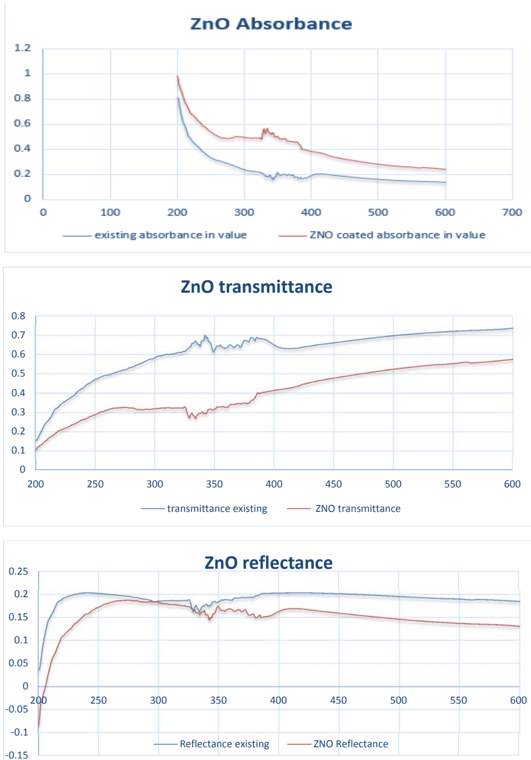
Figure-4. Optical properties of coated solar cell a) Absorbance b) Transmittance c) Reflectance.
