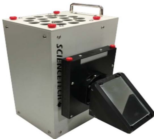
Figure-5. Solar Simulator [13].
