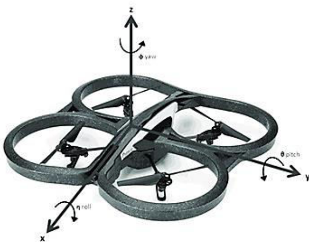
Figure-4. AR. Drone 2.0 with their respective axes.
