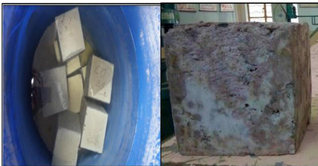
Figure-23. Curing of MgSO 4 cubes and specimen of MgSO 4 cubes.
