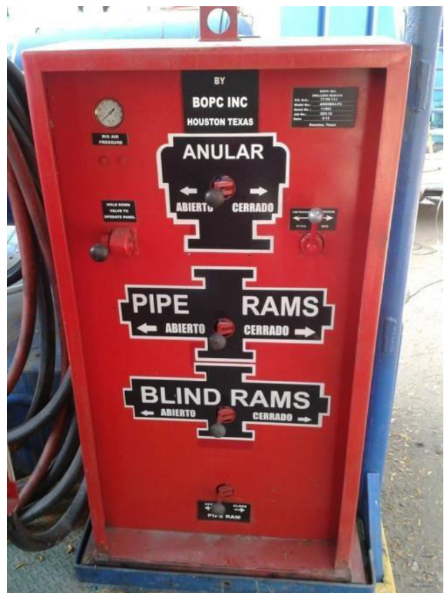
Figure-3. The basic control system of the 11983 accumulator.
