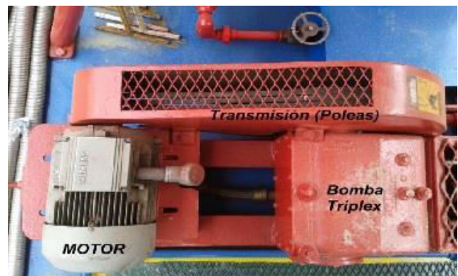
Figure-4. Electric motor connected to triplex pump.
