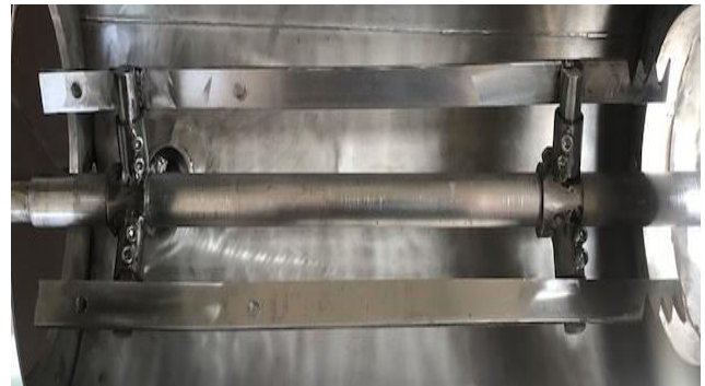
Figure-5. Shaft and beater blades mechanism of fruit pulp processing unit.
