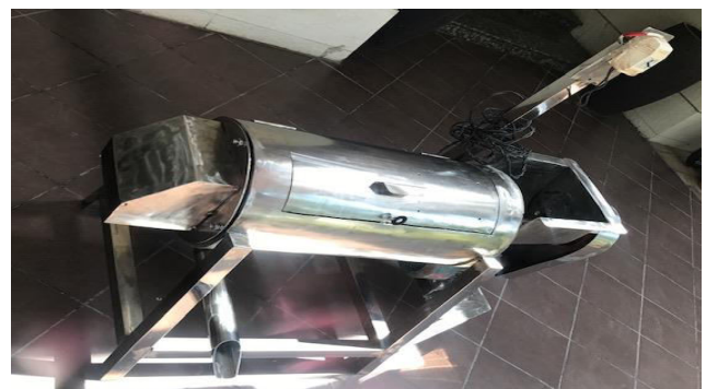
Figure-6. Fabricated stainless steel fruit pulp processing unit.
