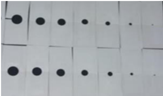
Figure-4. Specimens with a combined defect after testing.
