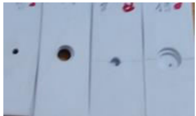
Figure-3. Rectangular specimens with a combined defect: hole plus single notch and hole plus double notch.
