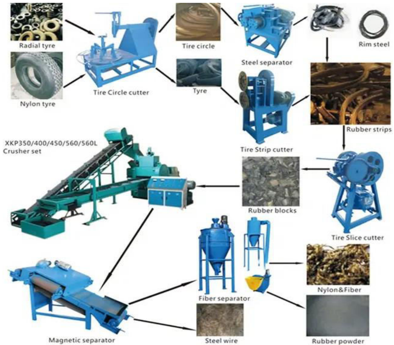
Figure-5. Process for obtaining rubber crumbs [17].
